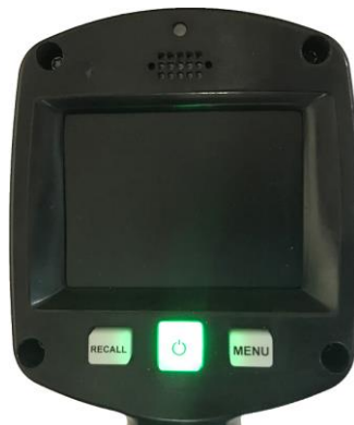
Figure 3.3b Power button illuminated when SVR3D is OFF and charging
